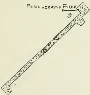
FIG. 132.—SECTION OF TILE SHOWING LOCKING PIECE
